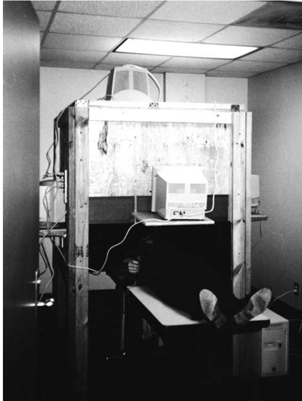
Figure 1. Physical display apparatus. Subject supine. Four of the six display monitors mounted to the walls of the node are visible.
